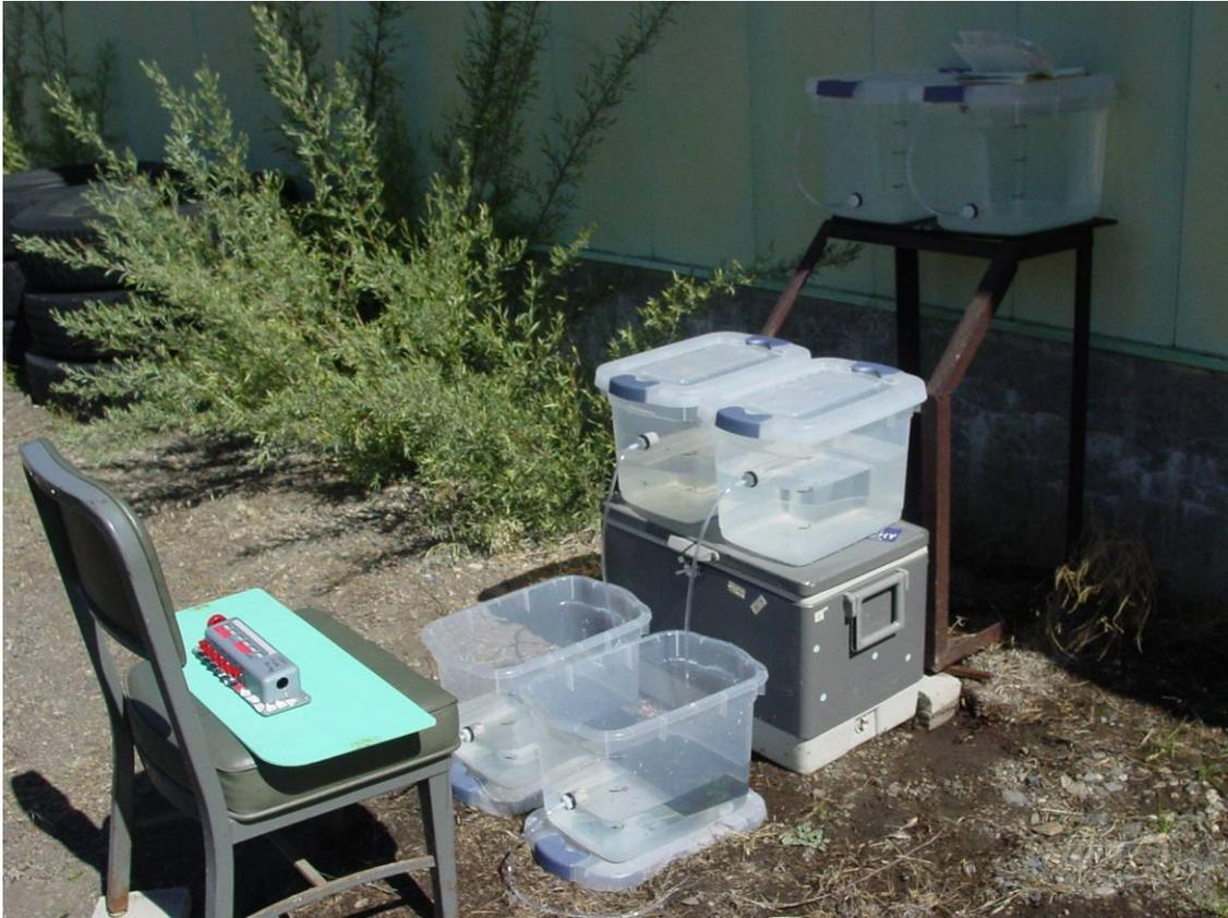
Figure 5. Gravitational flow-through system used in antipredator response experiments
