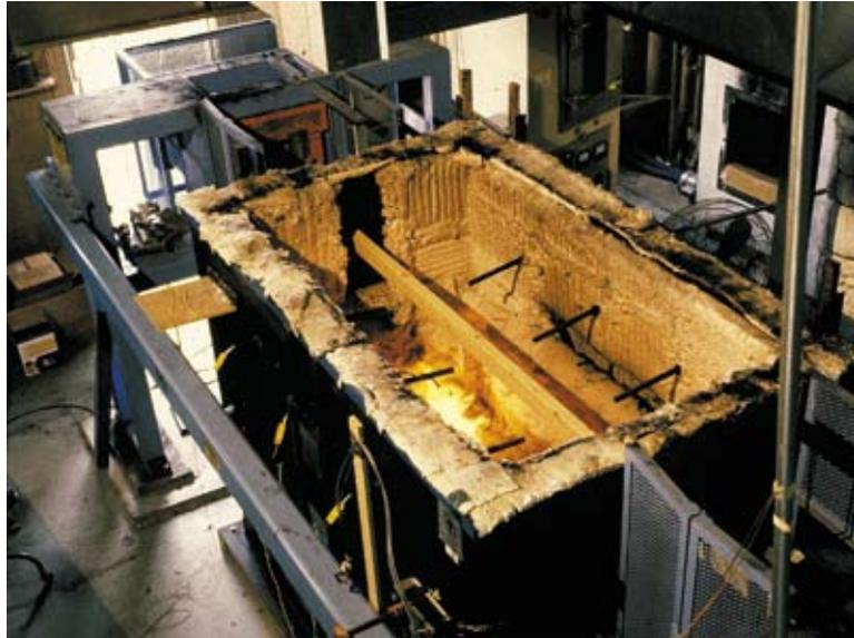
The FPL 1.2- by 1.8-m horizontal furnace and tension apparatus (ASTM E 119 fire-exposure equipment) can be used as (1) a horizontal furnace to test a panel product for fire penetration or (2) a tension apparatus to test a wood member simultaneously exposed to fire and tensile load.
