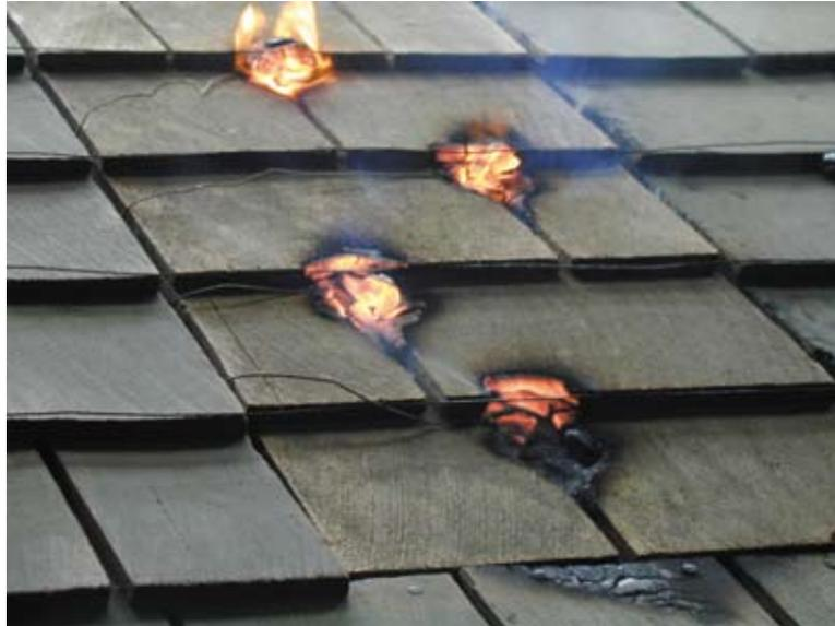
Testing a fire-retardant treatment with ASTM E 108 Class C burning brands.
