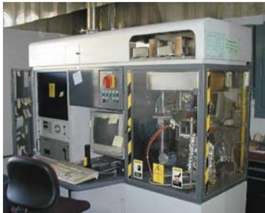
Present-day cone calorimeter (ASTM E 1354) that uses the oxygen consumption method to measure heat release rate.
