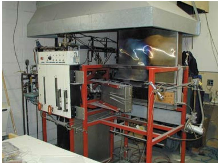
One of our small-scale tests is the Lateral Ignition Flame-Travel (LIFT) apparatus (ASTM E 1317 or E 1321).
