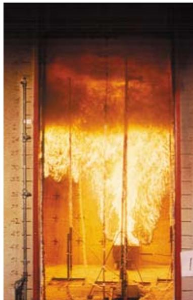
Small-scale tests are used to predict time for flashover in full-scale room/corner test (ASTM E 2257).
