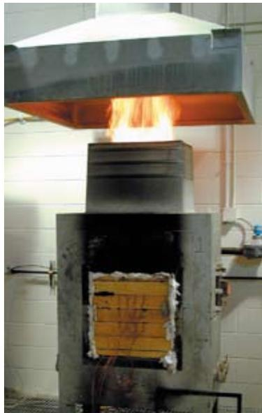
The FPL 510- by 510-mm small vertical furnace used to determine the charring rate of wood products subjected to the standard ASTM E 119 fire exposure.
