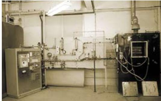
Original FPL heat release rate apparatus.
