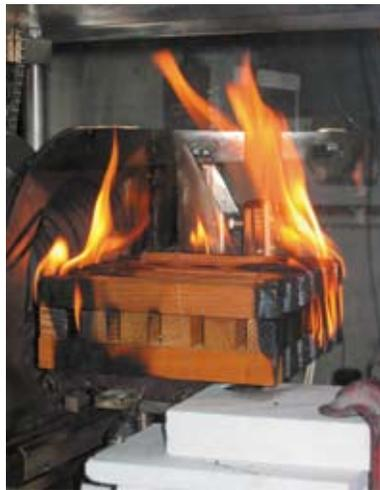
As part of the EcoSmart project, we have determined the heat release rate of the Class B brand that is used in the ASTM E 108 test for roof coverings.
