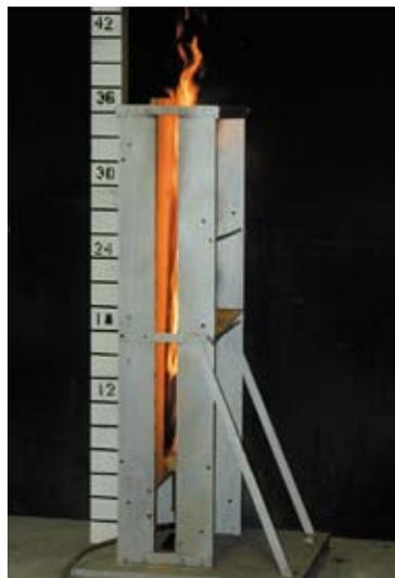
FPL-modified Schlyter panel test apparatus.
