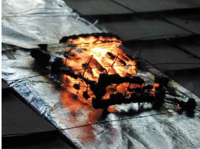
FPL is investigating the potential use of Forest Service emergency tent fabric to provide temporary protection to wood structures such as this ASTM E 108 Class B burning brand on wood shingles.
