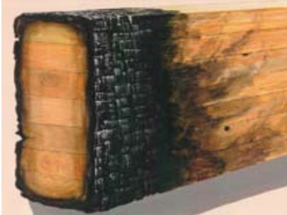
Fire resistance is largely a function of rate of charring and dimensions of the member.
